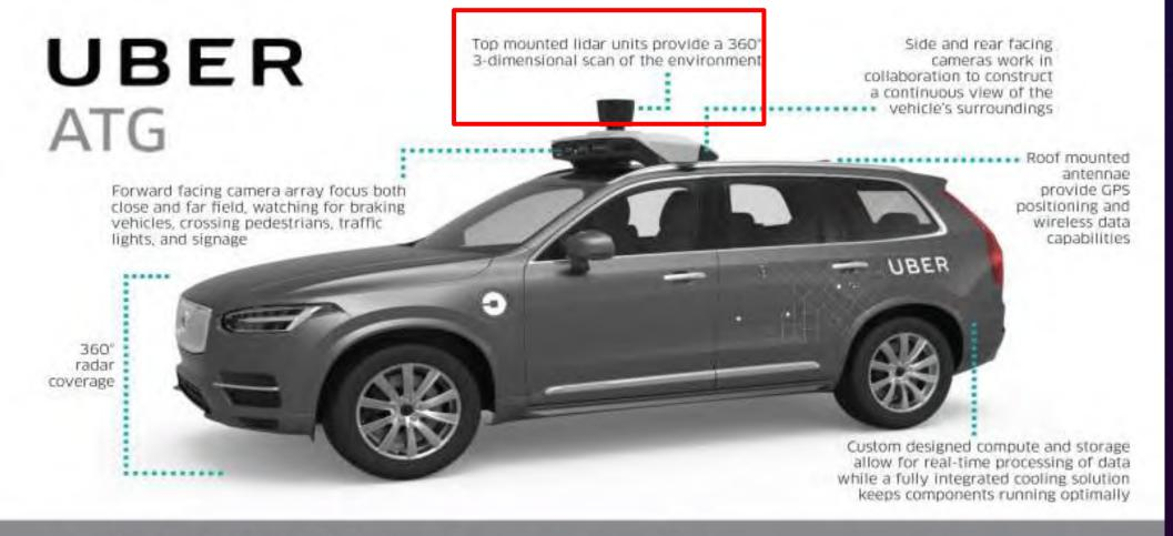
7 Cameras 1 Laser Inertial Measurement Units Custom compute and data storage 360° radar coverage
